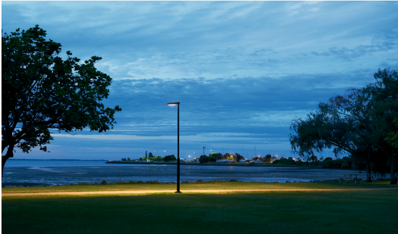
[P65] Ideal for the lighting of pedestrian and bicycle lanes to EN DIN 13201, Class S2-S4. Typical spacing between luminaires, 5 to 7 times the mounting height.
