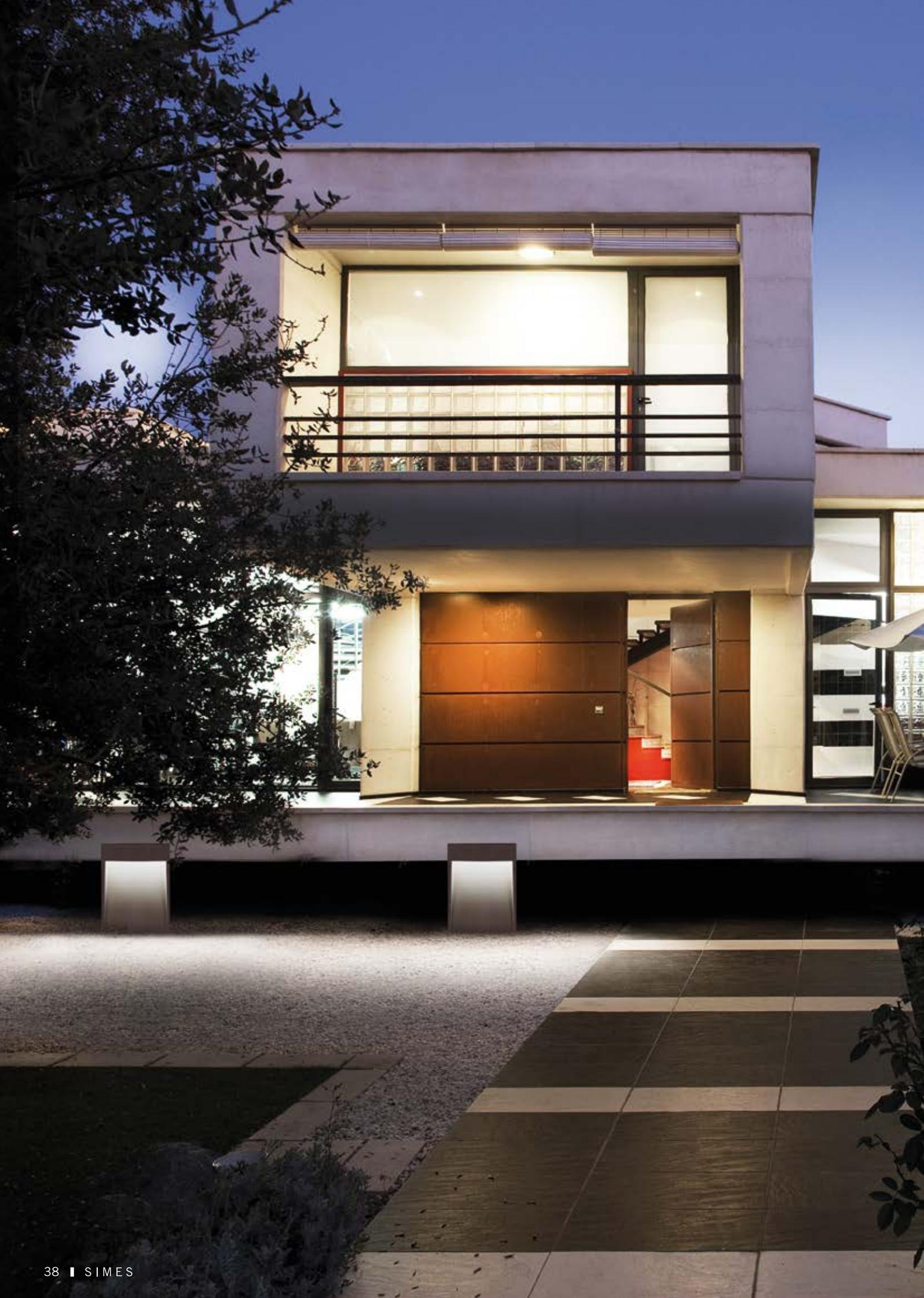
Concrete covering with added synthetic fibers with high mechanical strength. Lighting fixture in die-cast EN AB-47100 aluminium (low copper content) housing with high corrosion resistance. Clear polycarbonate diffuser. Stainless steel screws. Luminaire hard wired with single neoprene cable with cable gland. Silicone gaskets.
